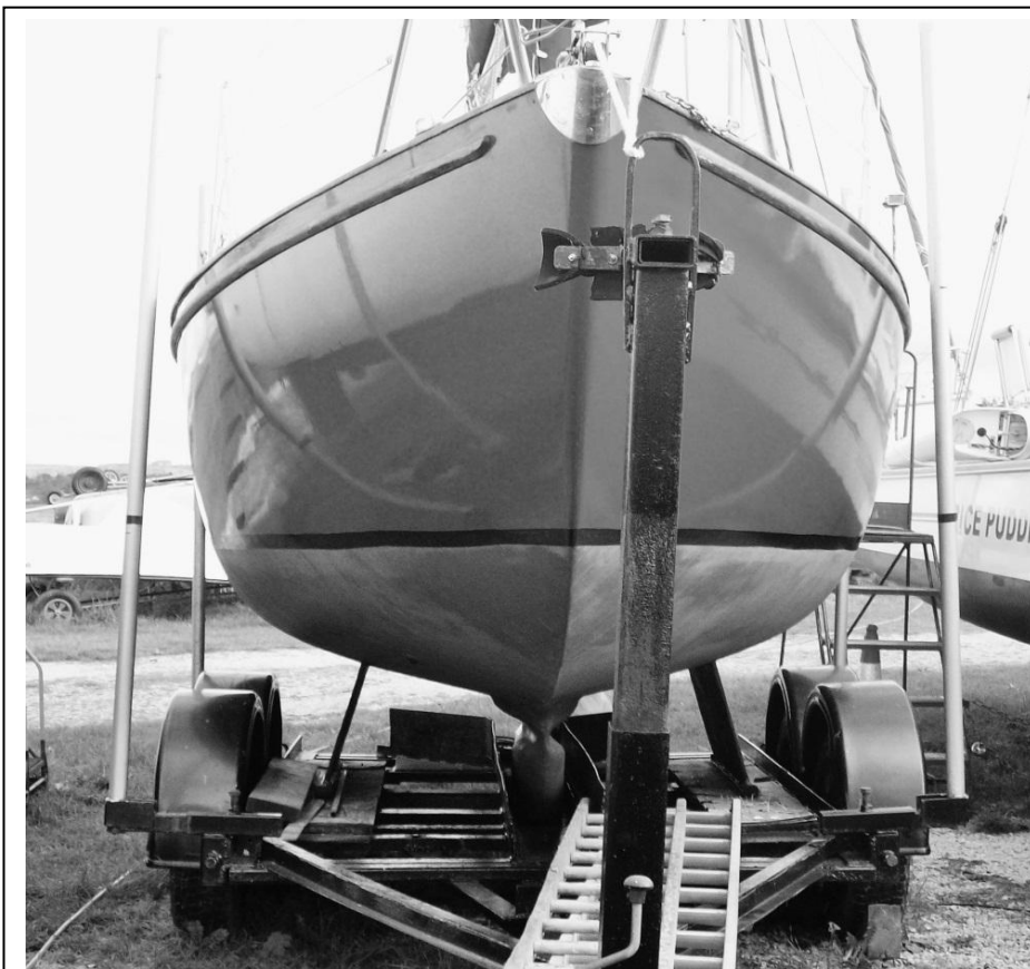
Docking arms show where the submerged trailer is lying and the stem post helps to locate Orla correctly fore and aft. Markings on the docking arm show when the falling tide has reached just the right level to float her onto the trailer. But immersion in seawater can increase trailer corrosion and damage brakes and wheel bearings. Hose down afterwards and service regularly.
