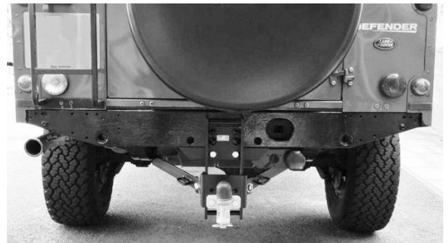
The drop plate on this Land Rover towbar allows the towball height to be adjusted to match the trailer hitch
