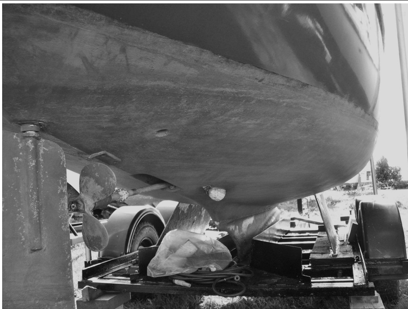
Orla's trailer has angled plates to guide the central ballast keel into position when floating her forwards onto the immersed trailer. The central keel is about an inch deeper than the bilge plates which are supported on wooden boards to make up the difference and keep the hull level.
