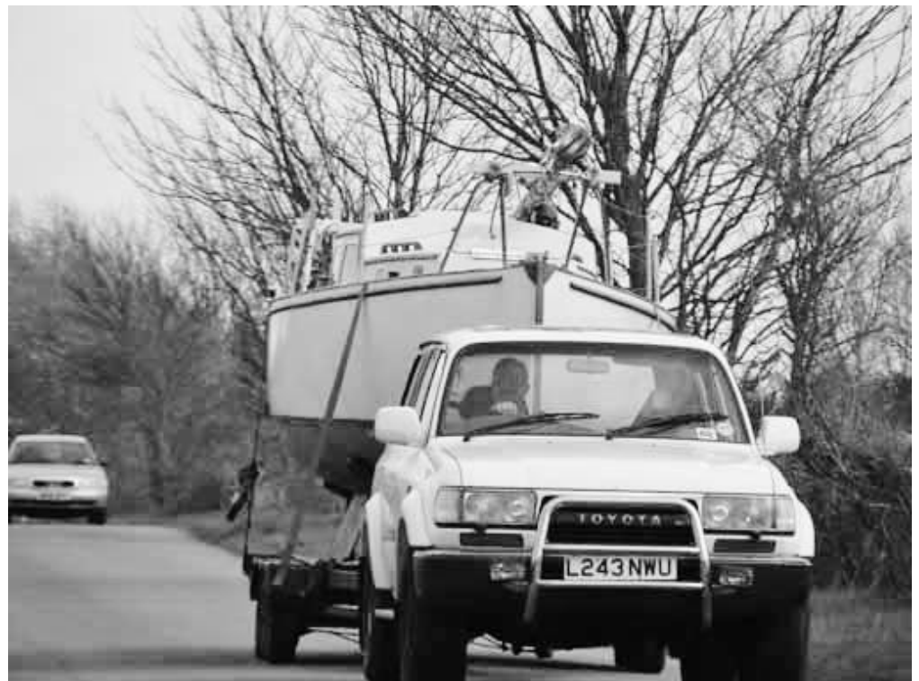
With an all-up weight for trailer and Trident likely to be around 2,500kgs, a substantial tow vehicle is needed and a 4-wheeled braked trailer
