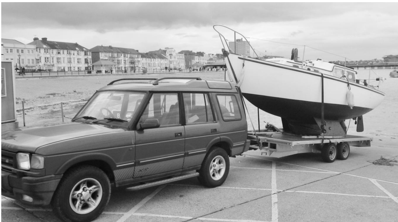
Four-wheel drive may be appreciated when negotiating weedy slips or rough ground. General purpose flatbed trailers need to be long enough to enable the Trident to be positioned forward in a nose-heavy position without hitting the towcar
