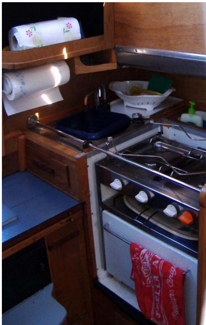
A neat set-up with both gimbaled alcohol stove and 'sink' to starboard leaving the port side chart table free. But for real minimalism, how about this flush-decked burner (below) with accessible stowage
