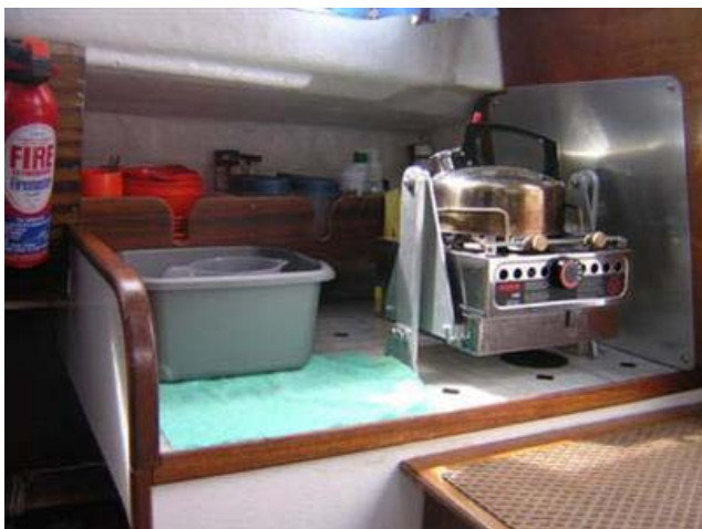
A neat set-up with both gimbaled alcohol stove and 'sink' to starboard leaving the port side chart table free. But for real minimalism, how about this flush-decked burner (below) with accessible stowage
