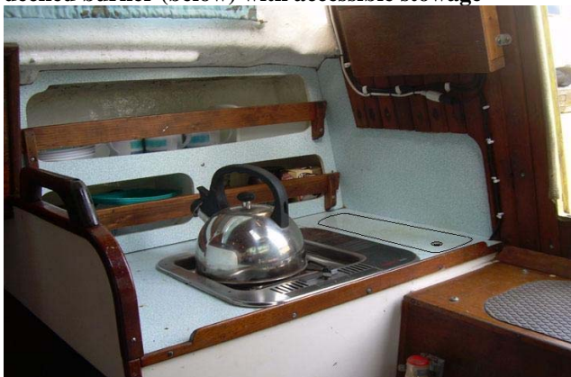
A neat set-up with both gimbaled alcohol stove and 'sink' to starboard leaving the port side chart table free. But for real minimalism, how about this flush-decked burner (below) with accessible stowage
