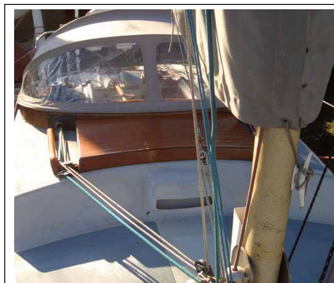
Pai Nai's hood bridge, hatch garage and lines led to mast
